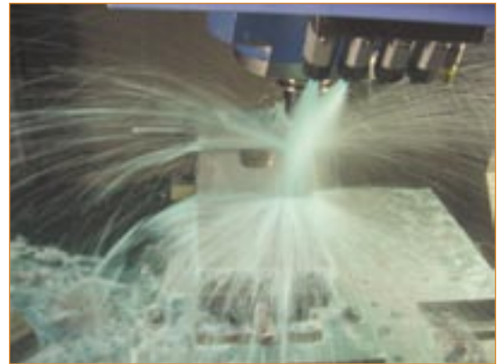
Ti5553 Forged Sample and (IMG-0787) fixtured in Mazak milling machine Credit: Teeter Marketing Services, LLC
